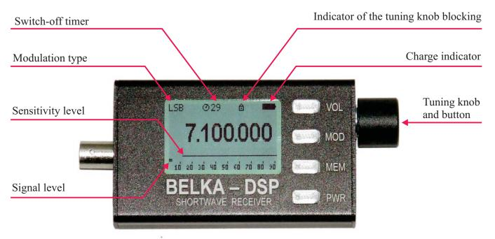
Radio receiver works in the frequency range 3.5-30 MHz. Input circuits of the radio receiver operate best with telescopic antenna of approximately 80 cm length.
