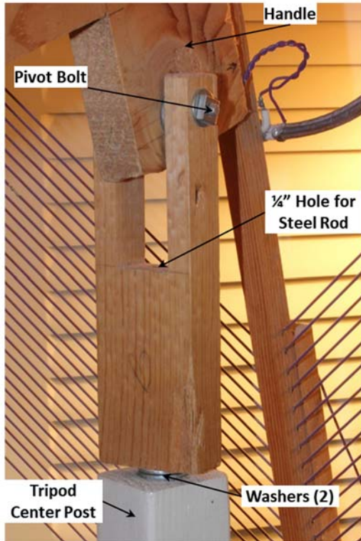
Figure 3-7. Universal Fork Installed
